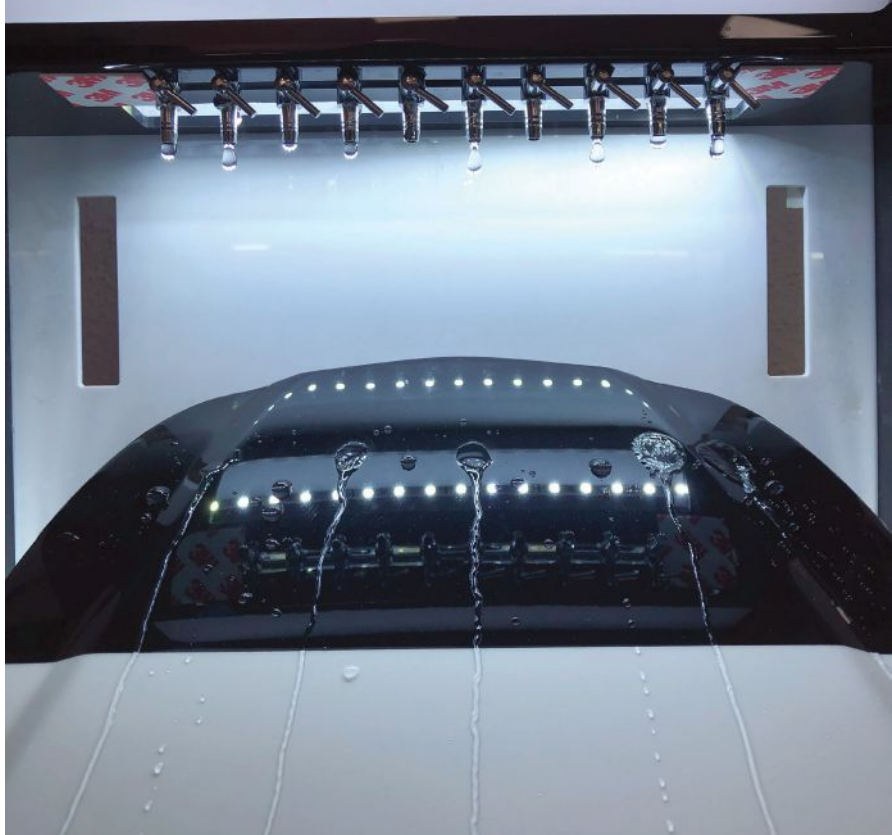
A water-dripping device that showcases a new hydrophobic PPF.
