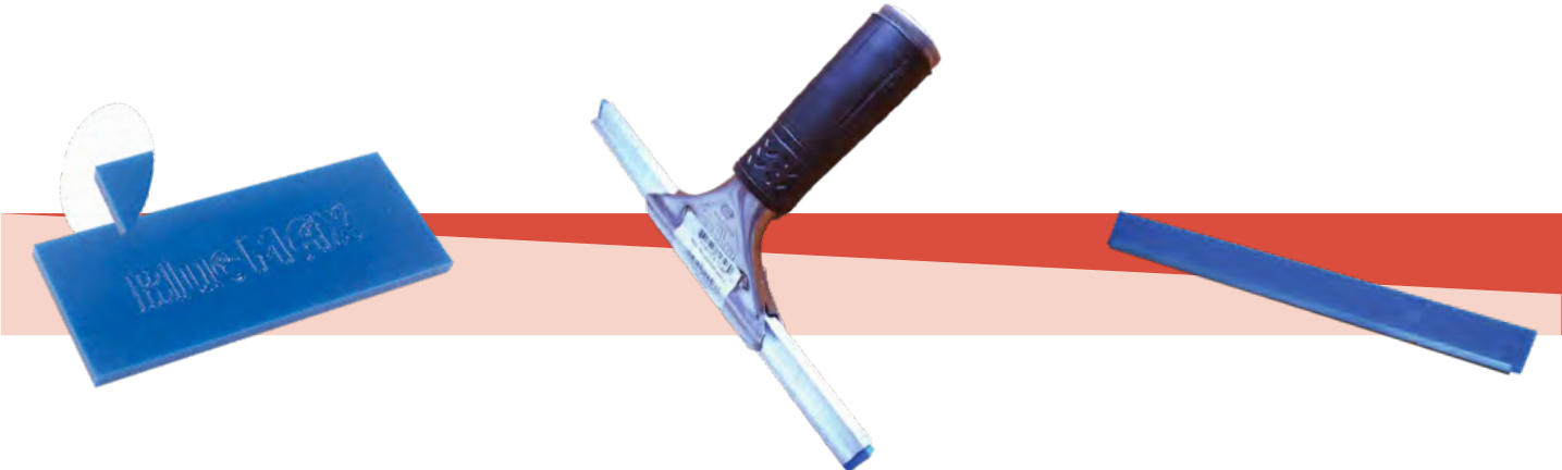
SMT-3223 | 5" BLUE MAX SQUEEGEE, SQUARE One of the basic tools of the window film professional. Blue Max can be used very well to remove large quantities of water during installation. The square-edged squeegee is even stronger, recommended specifically for safety films
